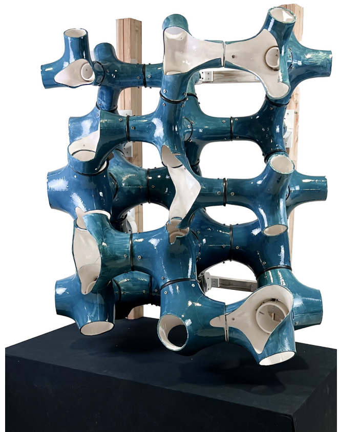
Figure 4. Ceramic multi-part assemblage prototype . MSD-RAS 2022-3 Spring Semester Project “Dynamic Slip-Casting”.
